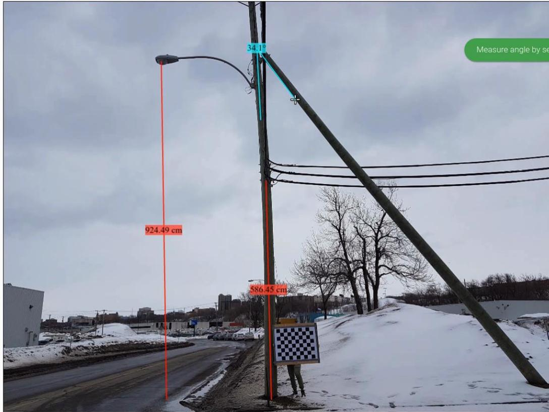
Measure angle by selecting three points sequentially
