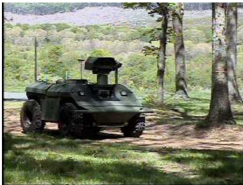
Figure 8: The GDRS eXperimental Unmanned Vehicle (XUV) used to acquire data for the experiments presented in this section.
