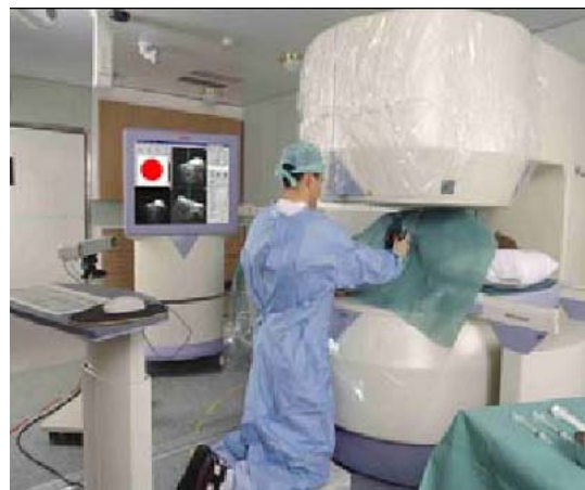
Figure 1. Open-field architectures of interventional magnetic resonance systems allowing horizontal and vertical access for imaging and image-guided interventions.
