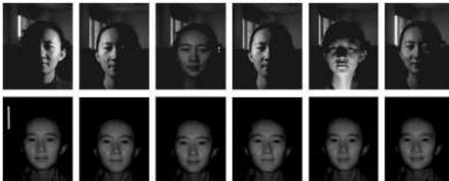
Figure 6. Visible images (top) and NIR images (bottom), we can see that NIR is less sensitive to illumination changes
