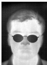
Figure 1. Thermal face image showing infrared opacity to eyeglasses
