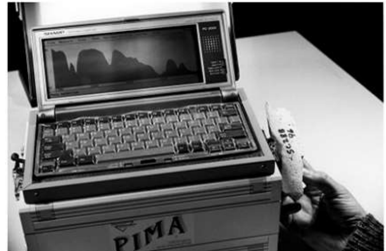
Photograph showing measurements being made with the PIMA II field spectrometer. Picture from: Kruse, F. A. (1996). Identification and mapping of minerals in drill core using hyperspectral image analysis of infrared reflectance spectra. International journal of remote sensing, 17(9), 1623-1632.
